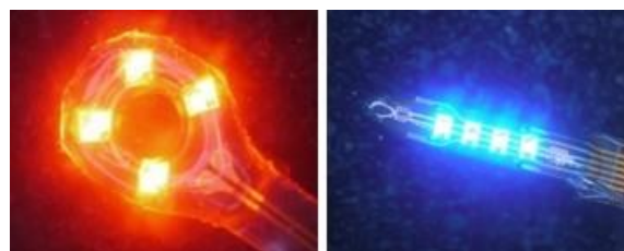
Fig 2. Micrographs of ring- (left) and linear-type (right) devices for stimulating neurons in transgenic rodents.
