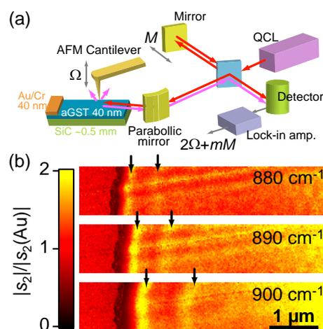
Figure 1 (a) Configuration of the s-SNOM setup. The scattering signal (pink arrows) is interfered with a reference light (red arrows). (b) Normalized near-field maps of the SPhPs excited at the gold edge with three different excitation frequencies.
