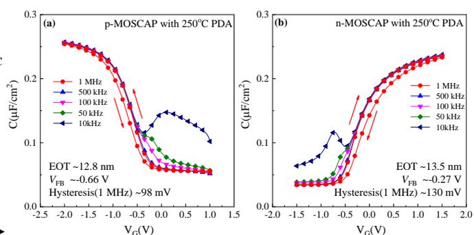
Fig. 2  $C-V$  characteristic of (a) p-MOSCAP and (b) n-MOSCAP fabricated under  $250^\circ\text{C}$ .
