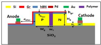
Figure 1: Schematic of Graphene based polymer filled silicon slot waveguide
