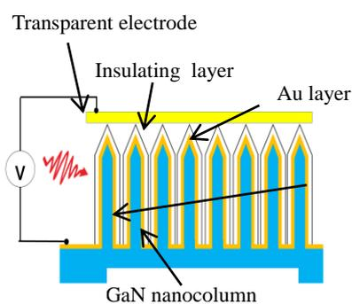
Fig. 1: Schematic of nanocolumn rectenna
