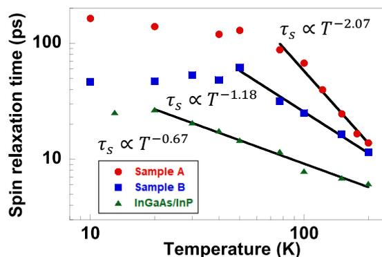
Fig. 2 Temperature dependences of the spin relaxation time for sample A (circle dots), sample B (square dots) and InGaAs/InP MQWs (triangle dots) at 30 mW.
