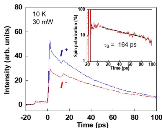
Fig.1 Time evolutions of spin-dependent reflection intensity for excitation power of 30 mW at 10 K in sample A. The inset shows the time evolutions of spin polarization.
