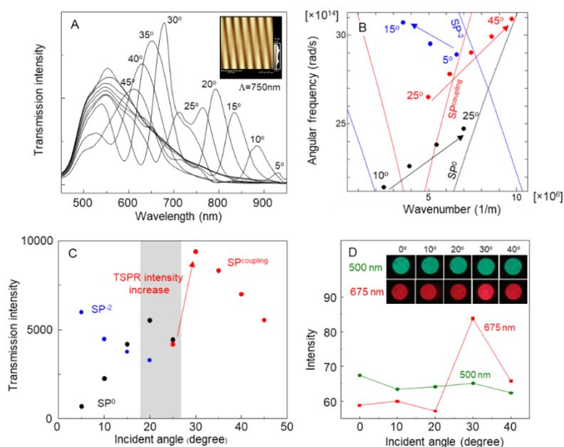
**Fig. 1** (A) TSPR spectra of gold-coated CYTOP grating substrate. (B) SP dispersion branch of conventional mode of  $SP^0$  (black) and  $SP^{-2}$  (blue) and SP coupling mode (red), experimental and calculated results are shown in dots and line, respectively. (C) TSPR intensity plots against the light incident angle. (D) Transmitted images and their intensities at the light incident angle from 0° to 40° and the wavelength of 500 nm (green) and 675 nm (red).
