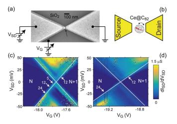
Figure 1. (a) Scanning electron micrograph of a electromigrated nanogap, where the position is indicated by the arrow.  $V_{SD}$  and  $V_G$  are source-drain voltage and gate voltage, respectively. (b) Schematic of the device structure of a Ce@C<sub>82</sub> single-molecule transistor (SMT). The dipole moment induced by the Ce atom in fullerene is denoted by red arrow. (c) and (d) Coulomb stability diagrams for the same SMT before and after the application of  $V_{SD} = 0.6$  V, respectively.
