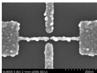
Figure 2: Typical SEM image for electrodes
