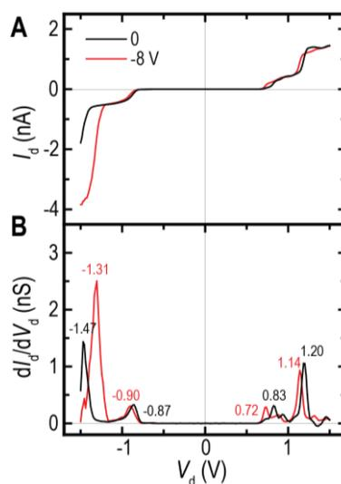
Figure 3:  $I$ - $V$  characteristics under the application of gate voltage of 0 and  $-8$  V at 9 K
