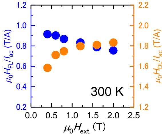
Figure: external field dependence of the SOT effective field per applied current at 300 K.
