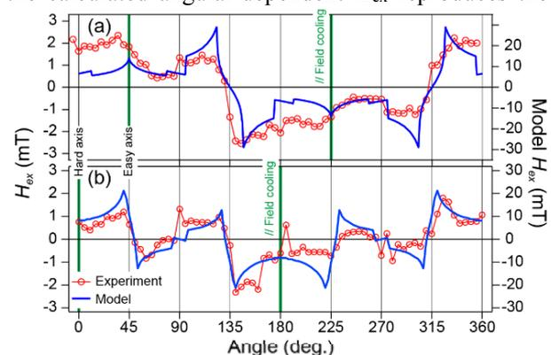
Fig. 1. Angular-dependent  $H_{\text{ex}}$  of (a) field cooling // easy and (b) // hard axes, respectively.
