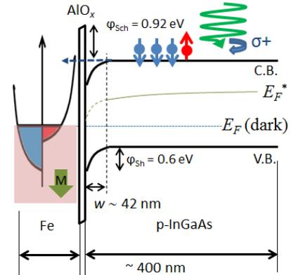
**Fig. 1:** Energy band diagram of the InGaAs active region of the refracting-facet spin-PD. Photogenerated spin-polarized carriers diffuse toward the p-depletion region. The built-in field inside the depletion region ballistically transports the electrons to the Fe/ $\text{AlO}_x$  junction where the electrons undergo spin-dependent tunneling.
