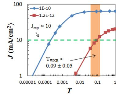
**Fig. 2:** Self-consistent solutions for the current  $J$  as function of  $T$  for  $\tau_{rec}^* = 1 \times 10^{-10}$  and  $1.2 \times 10^{-12}$  s.
