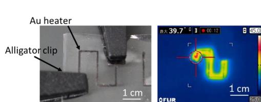
Fig. 1 Optical and IR photo of the heater
