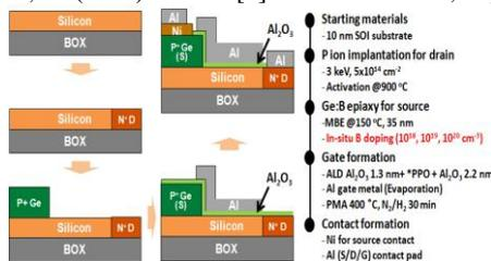
Fig. 1 Process flow of the Ge/Si TFETs
