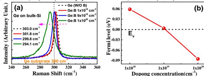
Fig. 2 (a) Raman spectra and (b) Fermi level in Ge
