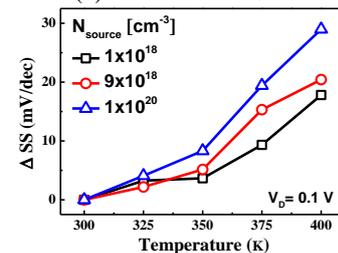
Fig. 5 SS increment vs Temperature
