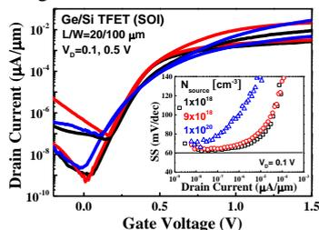
Fig. 3  $I_D$ - $V_G$  and curves of fabricated devices
