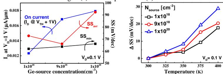
Fig. 4  $I_{on}$  and SS vs  $N_{source}$
