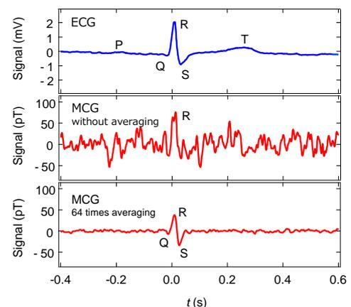
Fig. 1 Electrocardiography (ECG) and magneto-cardiography (MCG) using TMR sensor.
