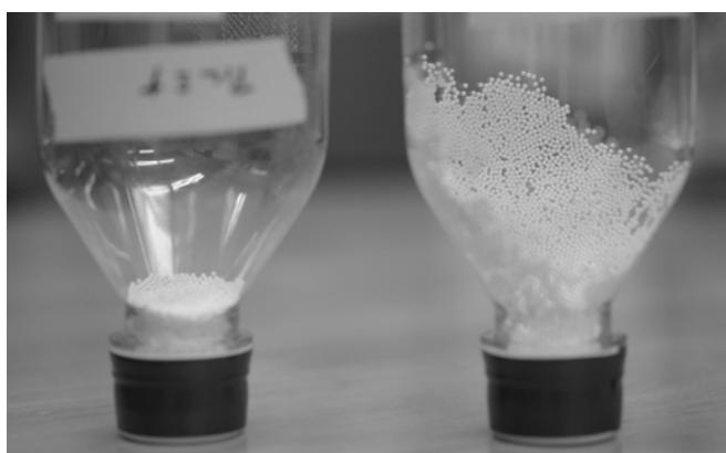
Fig. 1 Results after shaking the PET bottles; they contain alumina balls (diameter = 0.5 mm) and were filled with Ar gas (left) and dry air (right).
