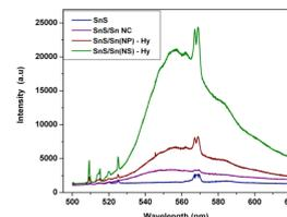
**FIGURE 2.** Photoluminescence spectra of SnS, SnS-Sn nanocomposites and SnS-Sn nano hybrids
