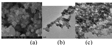
**FIGURE 1.** a) FESEM Image of SnS nanoparticles (b) SnS nanoparticles (c) HRTEM image of Sn hybrids
