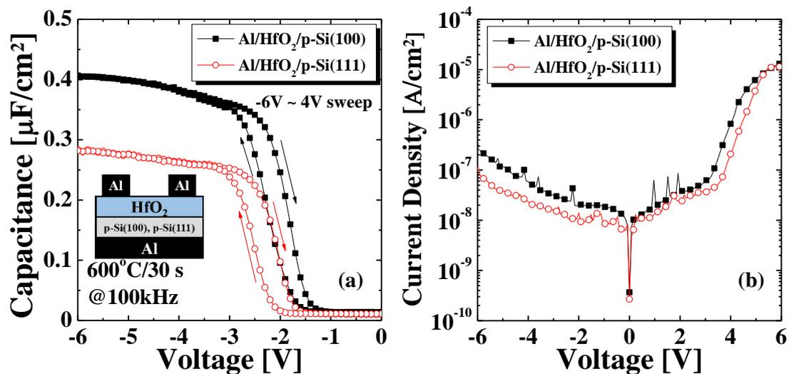
Fig. 1. (a) C-V and (b) J-V characteristics of the Al/HfO<sub>2</sub>/p-Si(100) and Al/HfO<sub>2</sub>/p-Si(111) diodes.
