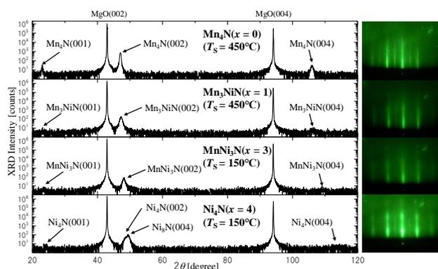
Fig. 1  $\omega$ - $2\theta$  XRD profiles and RHEED patterns observed along MgO[100] azimuth.
