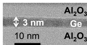
Fig. 2 XTEM of ultrathin GeOI channel fabricated with HELLO technology.
