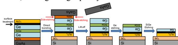
Fig. 1 Schematic flows of Hetero-Layer-Lift-Off (HELLO) technology for fabricating UTB GeOI substrates.
