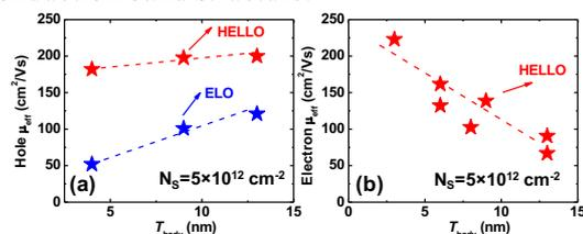
Fig. 3 (a)  $T_{\text{body}}$  dependence of effective hole mobility at  $N_s$  of  $5 \times 10^{12} \text{ cm}^{-2}$ , (b)  $T_{\text{body}}$  dependence of effective electron mobility at  $N_s$  of  $5 \times 10^{12} \text{ cm}^{-2}$ .
