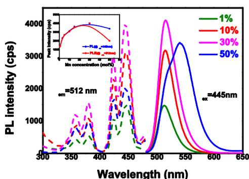
Fig 1. PLE and PL spectrum of 1, 10, 30, 50 mol% Mn-doped  $\gamma$ -AlON: Mg<sup>2+</sup>, Mn<sup>2+</sup>. PL intensity as a function of Mn doping amount is inset.
