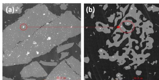
Fig 2. Cross-sectional SEM images of (a) 1mol% (b) 30 mol% Mn doped  $\gamma$ -AlON: Mg<sup>2+</sup>, Mn<sup>2+</sup> phosphor
