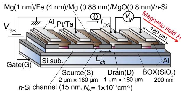
Fig. 1 Schematic illustration of our spin MOSFET and the measurement setup.
