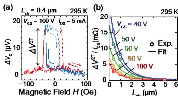
Fig. 2 (a) Spin-valve signal obtained in the sample with  $L_{ch} = 0.4 \text{ }\mu\text{m}$  and  $V_{GS} = 100 \text{ V}$ . (b)  $L_{ch}$  dependence of the spin-valve signal with various gate voltages  $V_{GS} = 40 - 100 \text{ V}$ .
