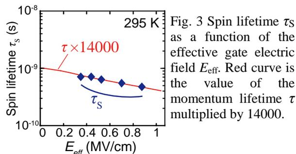
Fig. 3 Spin lifetime  $\tau_s$  as a function of the effective gate electric field  $E_{eff}$ . Red curve is the value of the momentum lifetime  $\tau$  multiplied by 14000.
