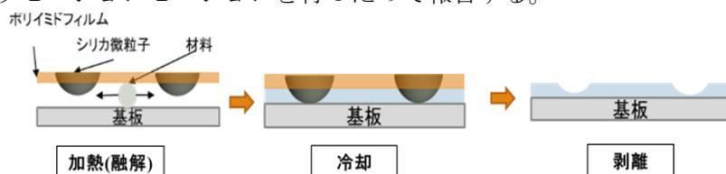
Fig. 1. Procedure of transfer-printing process.
