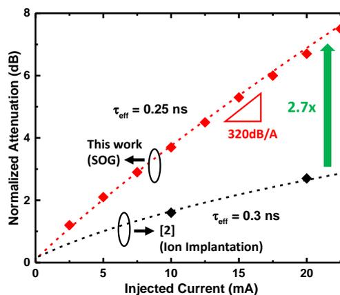
Fig. 2 Attenuation in Ge VOAs as a function of injected current.
