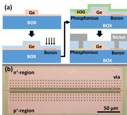
Fig. 1 (a) Process flow of a Ge VOA fabricated by SOG; (b) Plane-view microscope image of a 250- $\mu\text{m}$ -long Ge VOA.
