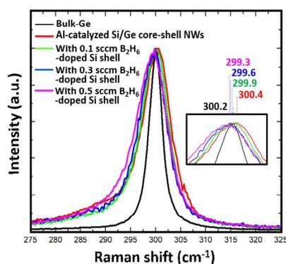
Fig. 2 Raman spectra of Ge optical phonon peaks of bulk-Ge, Al-catalyzed SiNW/Ge core-shell structure, and Al-catalyzed SiNW/Ge/B-doped Si core-double shell structures with various B<sub>2</sub>H<sub>6</sub> flow rates of 0.1, 0.3, and 0.5 sccm in outermost Si shell.
