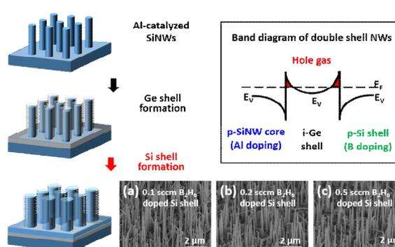
Fig. 1 Schematic, band diagram, and SEM images of Al-catalyzed SiNW/Ge/B-doped Si core-double shell formation with various B<sub>2</sub>H<sub>6</sub> flow rates of (a) 0.1, (b) 0.3, and (c) 0.5 sccm in outermost Si shell.
