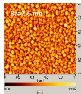
Fig. 1.  $1 \times 1 \mu\text{m}^2$  AFM image of the Al layer on the SiC substrate.
