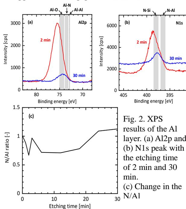
Fig. 2. XPS results of the Al layer. (a) Al2p and (b) N1s peak with the etching time of 2 min and 30 min. (c) Change in the N/Al
