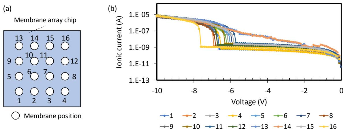
Fig. 1 Nanopore generation by dielectric breakdown technique for all 16 membranes using proposed 16-channel flow cell. (a) Schematic of membrane position. (b) Measured ionic-current during dielectric breakdown of each membrane.
