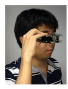
Fig.1 shows our holo-HMD, which is a monocular system[1]. The size is 90mmx130mmx30mm, and the weight is 120g, the visual field is 8 degrees.
