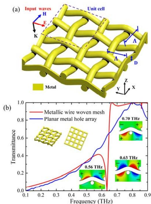
Fig. 1. 3D structure of MWWM. (b) Transmittance spectra of MWWM and planar metal hole array. (inset) THz field distributions in X-Z plane at 0.56, 0.63 and 0.7 THz.
