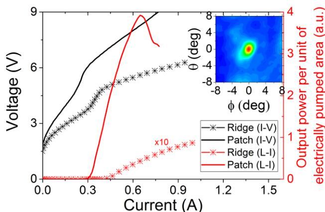
Figure 1. L-I-V characteristics of a DM ridge waveguide compared with the PAM array. Inset: measured far-field pattern of the PAM array. A beam divergence with FWHM=  $2^\circ \times 2^\circ$  was measured.
