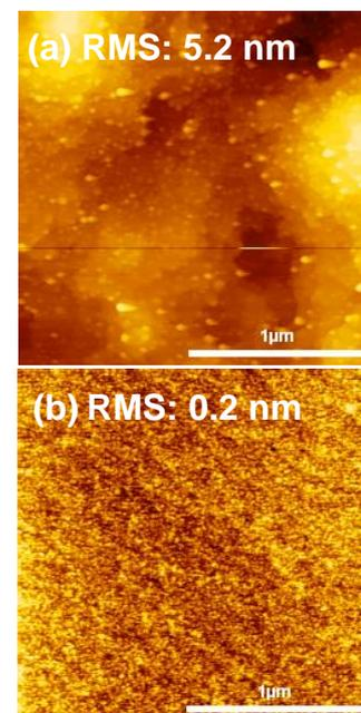
Fig. 1 AFM images of 1 nm-thick InN films on AlN templates (a) A and (b) B.
