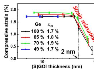
Fig. 3  $t_{\text{SGOI}}$  dependence of  $\epsilon_c$
