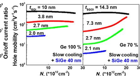
Fig. 5  $t_{\text{SGOI}}$  dependence of  $\mu_h$  as function of  $N_s$  to strained (S)GOI MOSFETs
