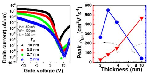
Fig. 4  $I_d$ - $V_g$  of ETB GOI pMOSFET, peak  $\mu_h$  and on/off ratio as function of  $t_{\text{SGOI}}$
