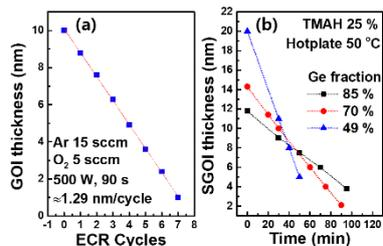
Fig. 1  $t_{\text{GOI}}$  as function of cycles (a)  $t_{\text{SGOI}}$  as function of etching time (b)
