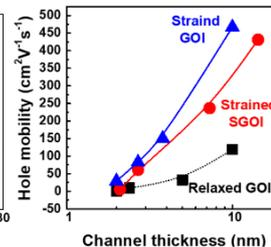
Fig. 6  $t_{\text{SGOI}}$  dependence of  $\mu_h$  degradation
