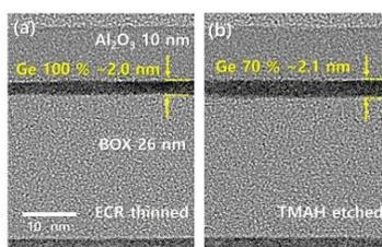
Fig. 2 TEM of ETB GOI 2 nm (a), and 2.1 nm (b)
