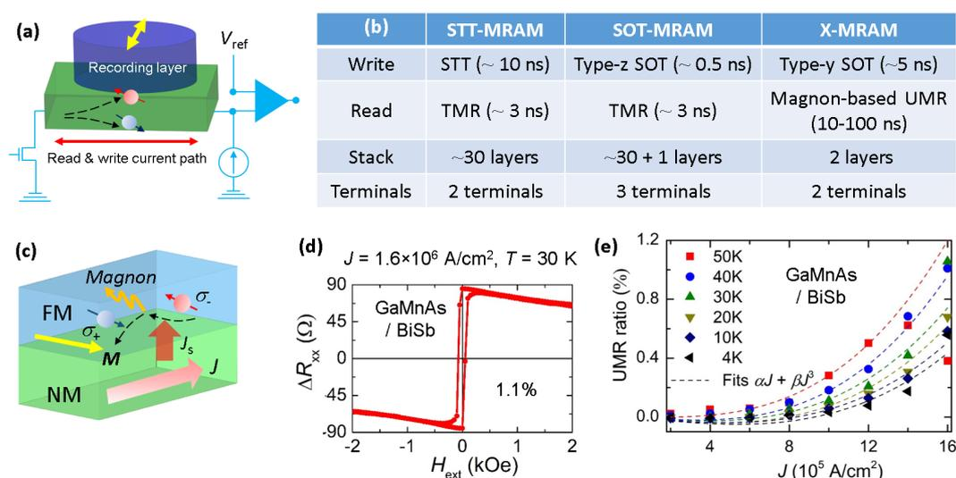
**Fig. 1.** (a) Schematic structure of X-MRAM. (b) Difference between STT-MRAM, SOT-MRAM, and X-MRAM. (c) Magnon emission/absorption and strong spin-disorder scattering mechanism for giant UMR. (d) Demonstration of a giant UMR of 1.1% in a GaMnAs/BiSb bilayer. (e) Temperature dependence of the UMR ratio of the GaMnAs/BiSb bilayer.
