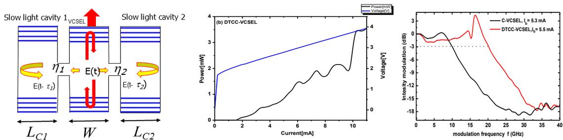
Fig.1. Schematic of DTCC-VCSEL Fig.(2) L-I curve for DTCC- VCSEL. Fig. 3. IM responses of C-VCSEL and DTCC-VCSEL.
