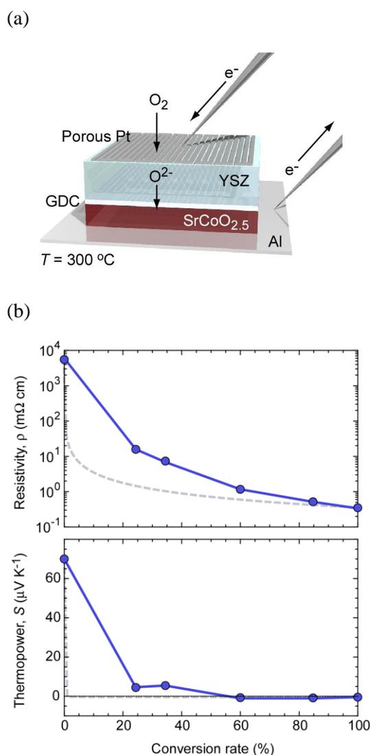
FIG. (a) Schematic illustration of the electrochemical oxidation of SrCoO<sub>2.5</sub> film grown on GDC-capped YSZ substrate. (b) Electron transport properties of the SrCoO<sub>x</sub> as a function of the conversion rate. The as grown sample (0 %) showed the resistivity of 5.5 Ω cm and the thermopower of +70 μV K<sup>-1</sup>, whereas 100 % converted sample showed 0.3 mΩ cm and -0.5 μV K<sup>-1</sup>. The dotted lines were calculated by assuming the electrical circuit was parallel.
