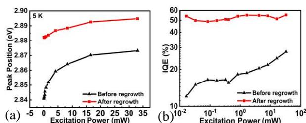
Fig.2. PL peak position as function of excitation-power (a) and IQE (b) of nanodisk before and after regrowth.
