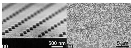
Fig.1. SEM of nanodisk before (a) and after (b) regrowth.
