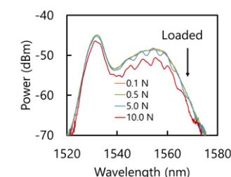
Fig. 3 Load dependencies of the reflected spectrum.
