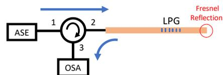
Fig. 1 Schematic setup of the cascaded LPG structure for strain and temperature sensing. ASE: amplified spontaneous emission, OSA: optical spectrum analyzer.
