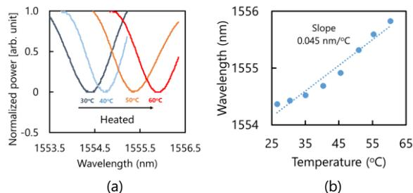
Fig. 4 Temperature dependencies of (a) the spectral dip and (b) its wavelength. The dotted line is a linear fit.
