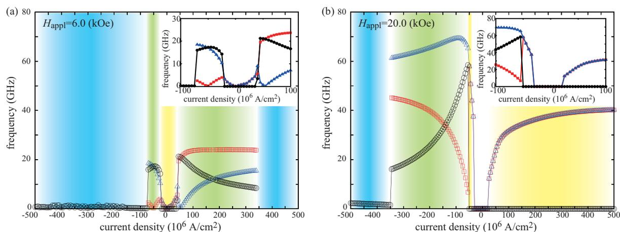
Figure 1: Current dependences of oscillation frequencies of magnetizations in the field-generation (red square) and spin-injection (blue triangle) in the presence of (a) small and (b) large perpendicular magnetic fields, respectively. The oscillation frequency of magnetoresistance is also shown (black circle).
