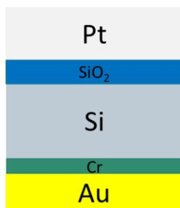
Fig. 1: Device structure
