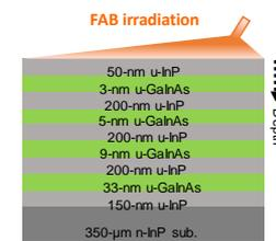
Fig. 2. Wafer structure.
