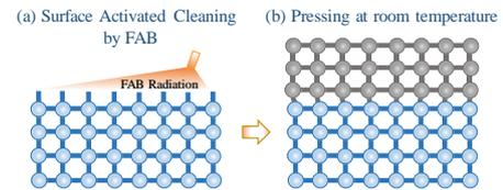
Fig. 1. Surface activated bonding using FAB.
