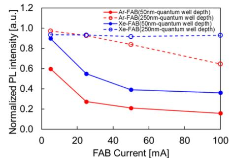
Fig. 3. FAB Current dependence of Normalized PL intensity at 50 nm and 250 nm-quantum well by Xe and Ar-FAB (FAB irradiation time: 10 sec).
