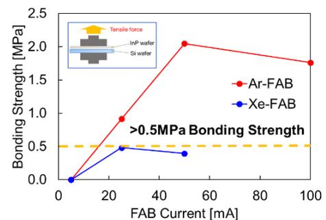
Fig. 4. FAB Current dependence of InP/Si Bonding Strength by Xe and Ar-FAB (FAB irradiation time: 10 sec).
