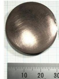
Fig. 1 Appearance of premix MVT bulk surface.
