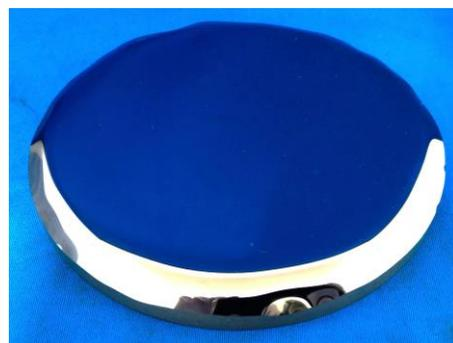
Fig.2 Photograph of  $\Phi 6$ inch 4H-SiC crystal by gas source method.
