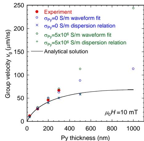
Fig.1 Summary of group velocity  $v_g$ . Red circles are experimental results and black solid line is the analytical solution. Blue and green are simulation results of ‘without conductivity’ and ‘with conductivity’, respectively.
