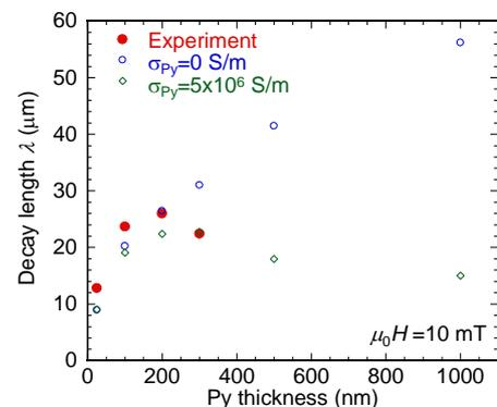
Fig.2 Summary of decay length  $\lambda$ . Red circles are experimental results. Blue and green are simulation results of ‘without conductivity’ and ‘with conductivity’, respectively.
