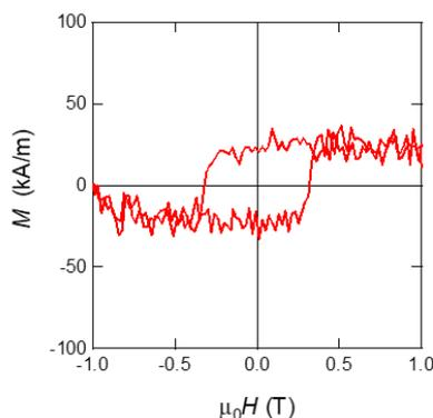
Fig. 1. Magnetization curve of CoGa/Mn/MgO structure measured at room temperature.
