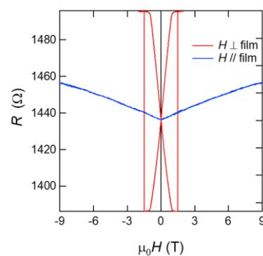
Fig. 2. Room temperature TMR curves with magnetic field ( $H$ ) for out-of-plane and in-plane
