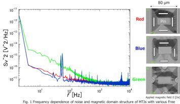
Fig. 1 Frequency dependence of noise and magnetic domain structure of MTJs with various Free layer shape: square (red), rounded square (blue), and side-notched square (green)
