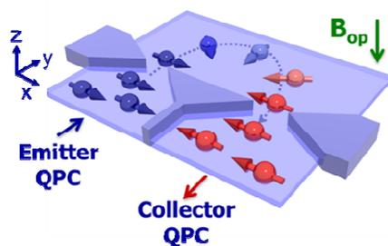
Fig. 1. Spin-momentum locked spin manipulation under transverse magnetic focusing.
