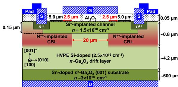
Fig. 1. Cross-sectional schematic of the vertical Ga<sub>2</sub>O<sub>3</sub> MOSFET. The aperture and source widths were 200  $\mu$ m.
