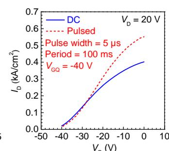
Fig. 3. DC and pulsed transfer curves of the vertical MOSFET.
