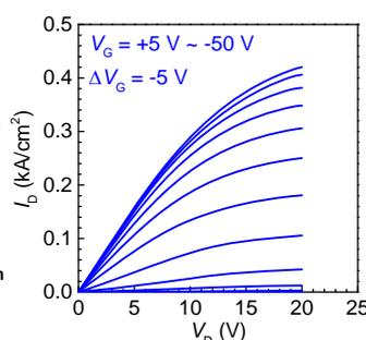
Fig. 2. DC output characteristics of the vertical MOSFET.
