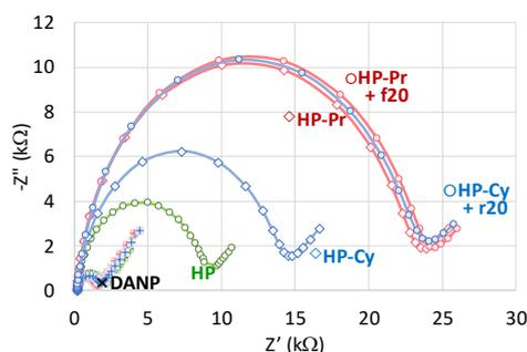
Fig 2. The Nyquist of HP-Cy, HP-Pr and after target DNA addition.
