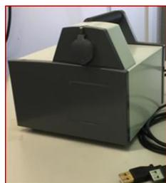
Fig.1 Appearance of a Compton camera
