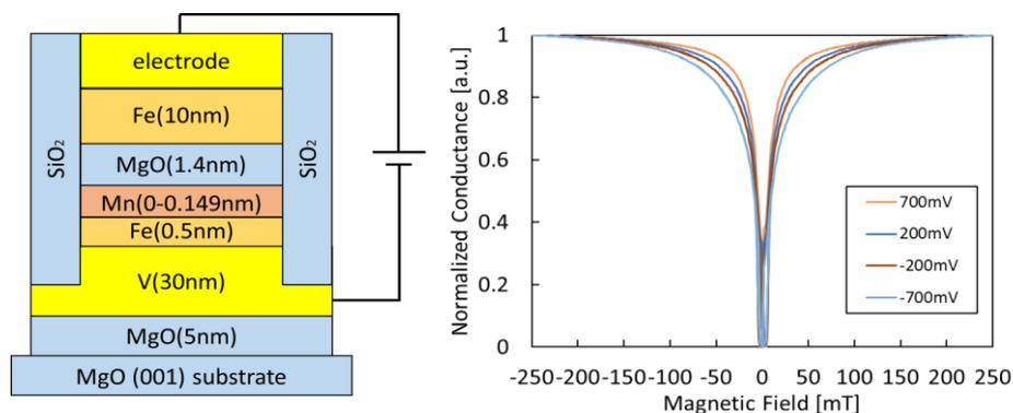
Fig.1 Multilayer structure      Fig.2 Normalized Conductance measured at various voltage
